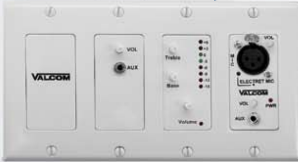
In-Wall Modular Mixer, w/Remote.....V-9985-W - 1 Mounts in 4 Gang Electrical Box • 6.64"W x 4.25"H x 2.0"D (16.87cm x 10.8cm x 5.08cm) 4.25 lbs (1.93 kg)
